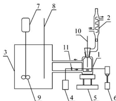
**Figure 1** Equipment for the measurement of solubility of benzoic acid derivatives in 1-octanol
